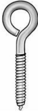
The “eye bolt” is a ½” lag eye screw, 6 inches long, with the shaft fully threaded. There is 4 inches of thread engaged in the wood beam. The beam is a variety of Douglas Fir.
