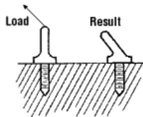
The load must be "in-line" with the axis of the eye, not perpendicular.
