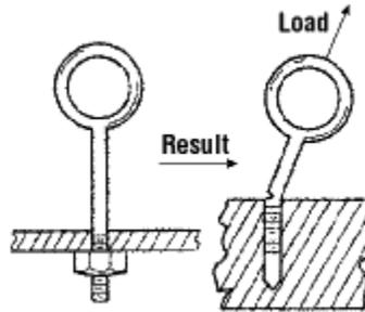
The shoulder on a shoulder bolt is meant to resist those lateral forces, to a degree. But only if loaded properly.
