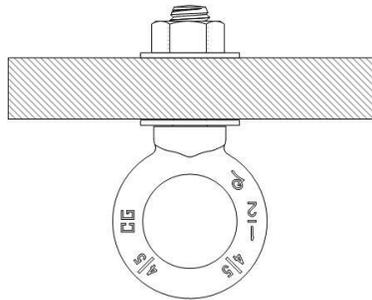
A ½” diameter eye bolt has a Working Load Limit (WLL) of about 2,600 lbs. with a 5:1 safety factor, giving a breaking strength of about 13,000 lbs. This is well over our design goal of 5,000 lbs.
